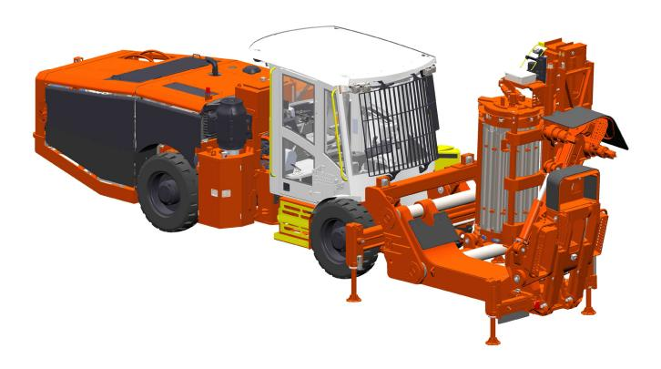
DU421-C is an ITH drill unitized with an on-board booster and complete with a FOPS/ROPS cabin. This drill is mounted on a mobile center articulated carrier designed for high mobility in underground mines with ramp access.
