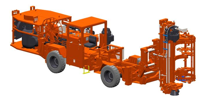
DU411 is an ITH drill unitized with an on-board booster. This drill is mounted on a mobile center articulated carrier designed for high mobility in underground mines with ramp access.
