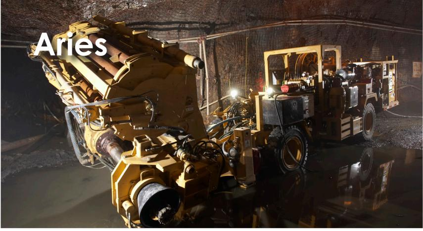
**Description:** The Aries drill is an ITH drill unitized with an on board booster. This drill is mounted on a mobile center articulated carrier designed for high mobility in underground mines with ramp access.
