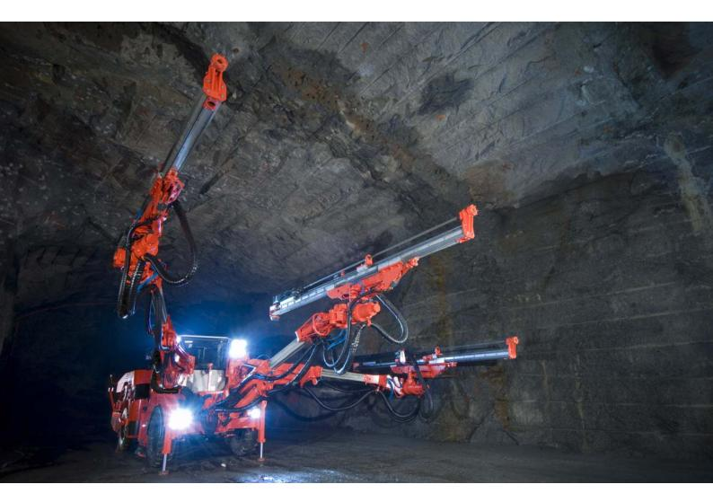
The Sandvik DT831-SC is a three boom electro hydraulic jumbo for fast and accurate drilling in tunneling and cavern excavation. The electronic controlled drilling system with added automatic functions and optional instrumentation enable productive and high quality excavation.
