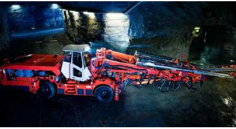
The Sandvik DT1231-SC is a 3-boom electro hydraulic jumbo for fast and accurate drilling in tunneling and cavern excavation. The advanced, electronic controlled drilling system with added automatic functions and optional instrumentation level enable productive and high quality tunneling.
