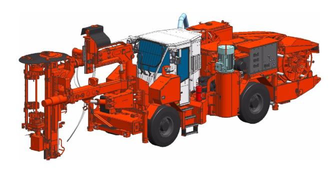
The Sandvik DS520-TC is a rock reinforcement drill rig specialized into cement grouted cablebolts installation. This rig is able to install up to 38 meters long cablebolts with several steel strand per hole.
