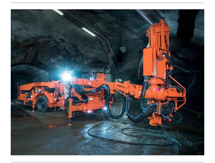
Sandvik DS511-C, equipped with Sandvik SB120S boom, offers the widest coverage currently available for underground mining operations and civil construction tunnelling.
