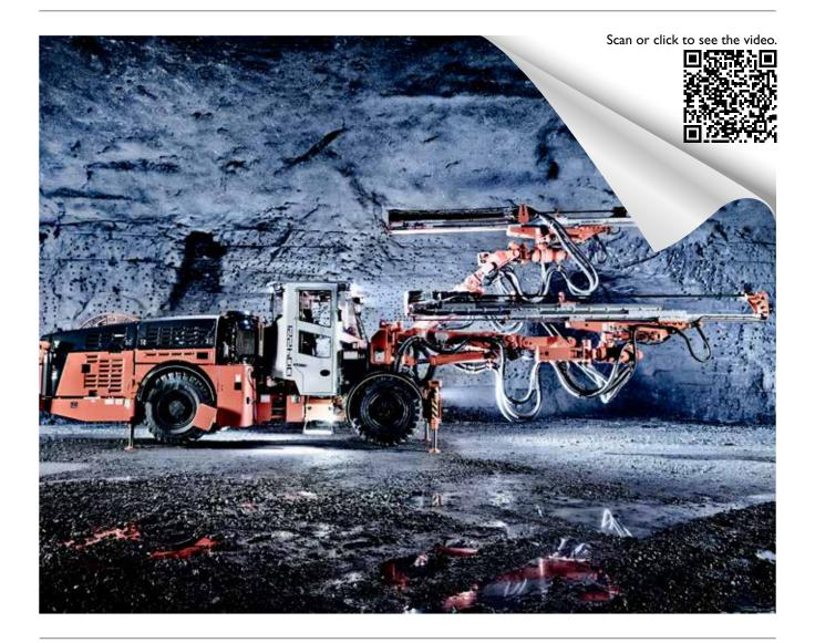
Sandvik DD422i is an advanced control system based electrohydraulic jumbo to provide top-level performance, accuracy and reliability for underground development drilling and small scale tunneling. The rig has the widest range of automatic drilling functions to give increased productivity with reduced costs, top-level product safety and access to the future of underground mining.
