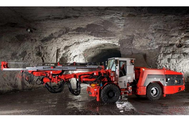
Sandvik DD421-60C is a two boom electro hydraulic jumbo for fast and accurate drilling in drifting and tunneling of 8-60 m<sup>2</sup> cross sections.
