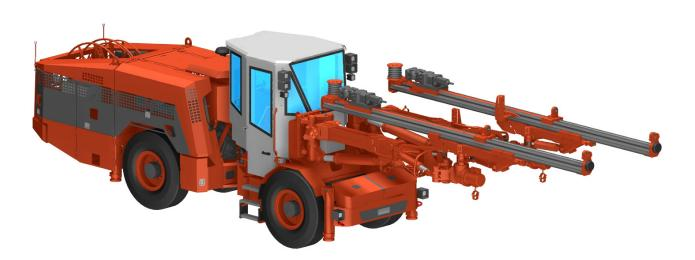
Sandvik DD321 is a compact two-boom jumbo for demanding conditions and multiple application. The jumbo is capable of face drilling, cross cut drilling and bolt hole drilling.
