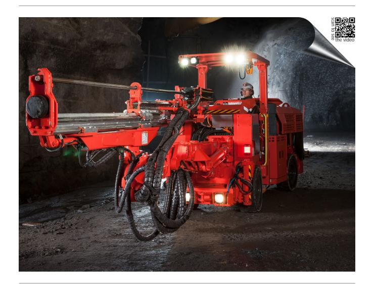
Sandvik DD211 is a single boom electro hydraulic drillrig for productive drilling in narrow vein applications.
