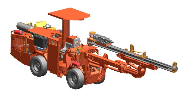
Sandvik DD210 is a compact and flexible single-boom electrohydraulic jumbo for tunneling and mining development in cross sections up to  $24\ m^2$ .
