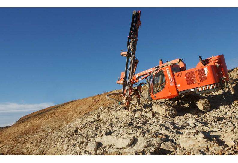
Sandvik DX800 is a hydraulic, self-propelled, self-contained, crawler based surface drilling rig equipped with a cabin (F.O.P.S. and R.O.P.S.) and rod handling system.
