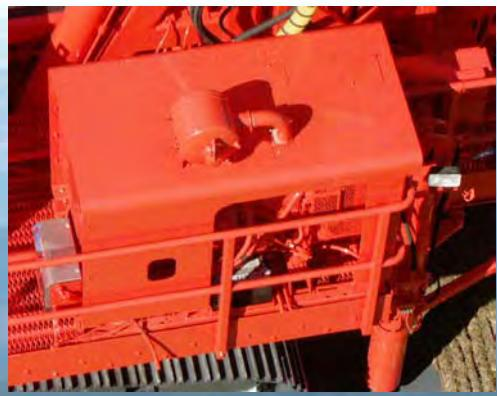
A **2,5 kW (34 hp) generator set** goes with special cold weather equipment and allows for shut-down and service in arctic conditions
